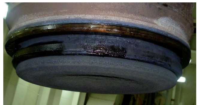
Fig. 3: Exhaust valve, S60MC-C8.1
